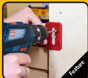
Drill guides for 5mm hole placement
