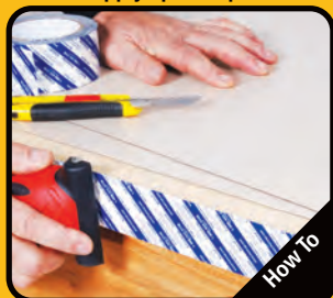
Roll for maximum adhesion
