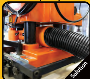
Attach a hose for quick clean up
